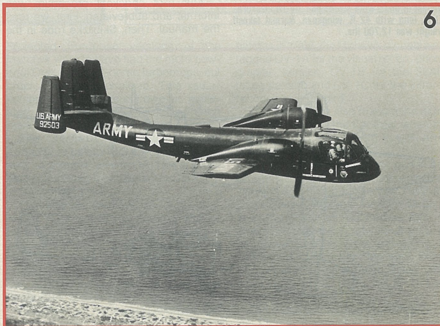
6. Clean production Mohawk in flight. AO-1AF (OV-1A) carried single KA-30 camera in fuselage. Camera could take pictures vertically or swivel 15 to 30 degrees, to either side, under control of pilot or observer. Production totaled 64 OV-1As.
