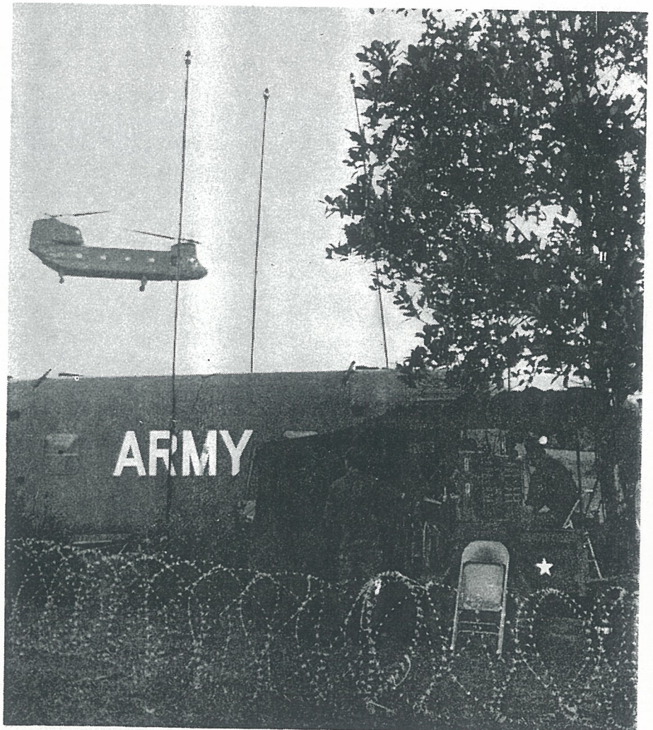
MOBILE SWITCHBOARD UNIT for telephone communications is set up on Special Forces airstrip during battle codenamed "Operation Masher." In background is Vertol Chinook.
