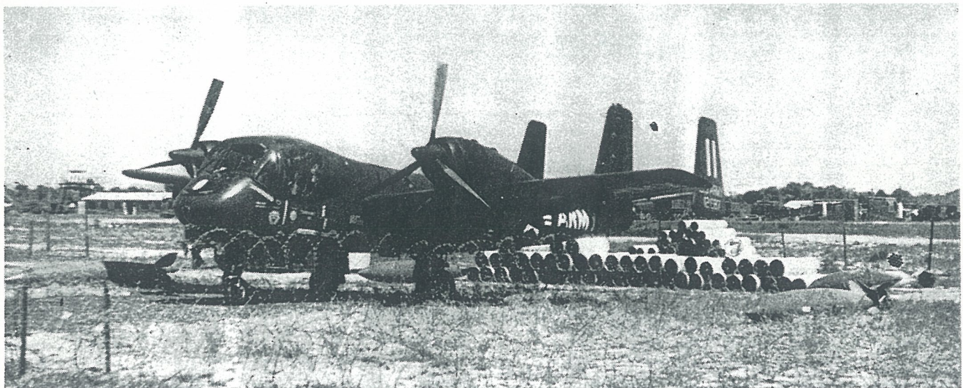
MOHAWK PARKED ON RAMP in South Vietnam is surrounded by barbed wire as a security measure. Other precautions include the use of expended rockets pods, stacked with sandbags piled on top. Note drop tanks on the ground nearby for quick attachment.
